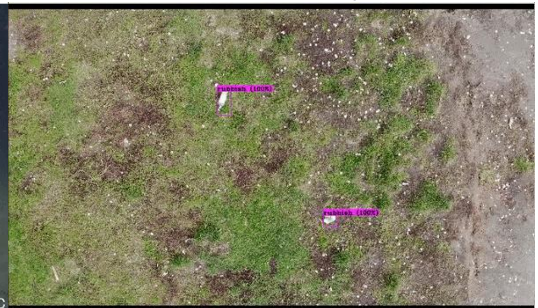
Autonomous, Onboard Vision-Based Trash and Litter Detection in Low Altitude Aerial Images Collected by an Unmanned Aerial Vehicle [Kraft et al., Remote Sensing 2021].
